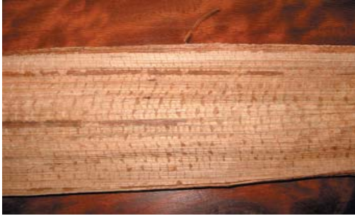
Banana fiber with inside (intestine layer) completely peeled
